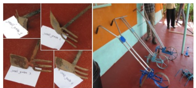
Figure 7: ROP Prototypes of two of the technologies: the “double jembe” and the wheel hoe
